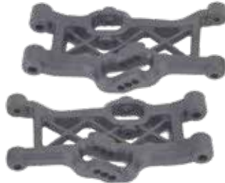
U8450 - Front Wishbones Stiff Flex (pr) U8451 - Front Wishbones Carbon Filled (pr)
